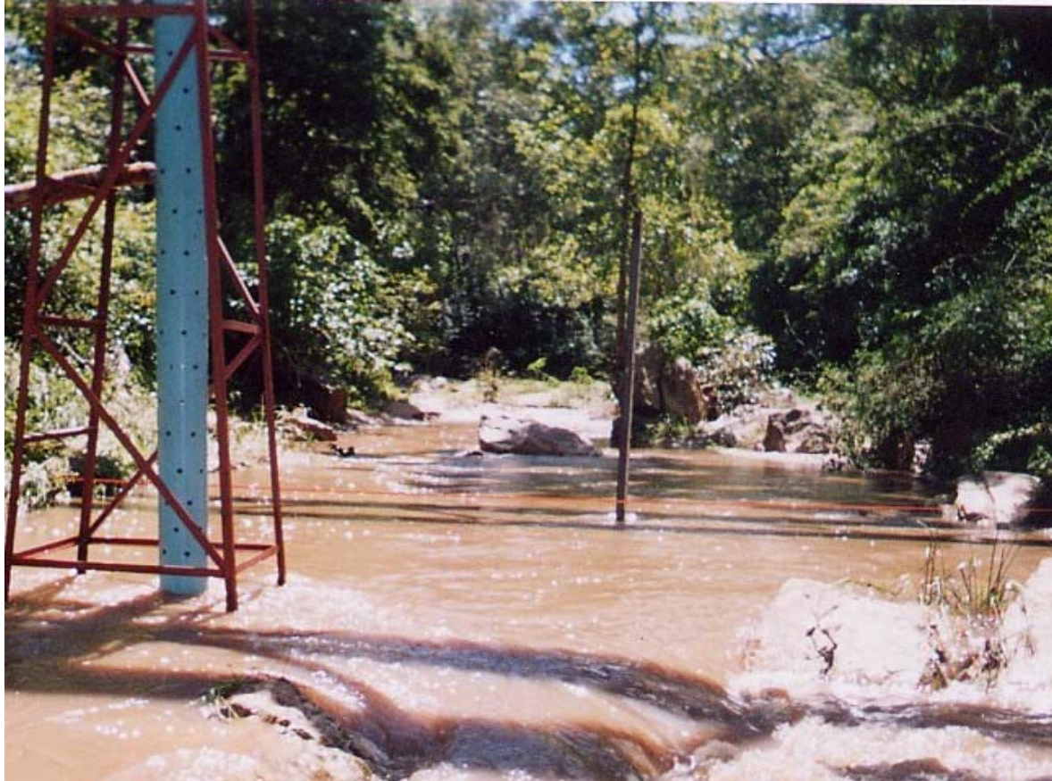
Figure 3-27. Stilling well and staff gauge in Hebbahalla control catchment
