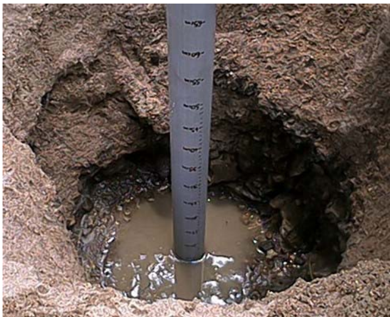
Figure 3-29. Instream shallow piezometer in Hediya degraded catchment
