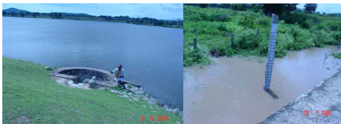
Figure 3-32. Monitoring of tank water level at sluice (L) and streamflow under bridge upstream of tank using staff gauge (R)
