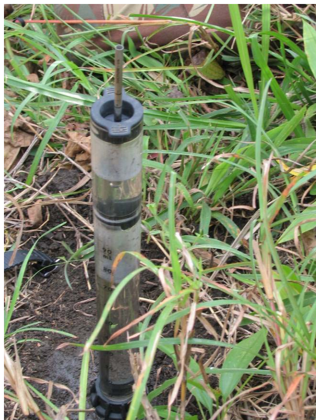
Figure 3-30. Disc permeameter for hydraulic conductivity measurements.
