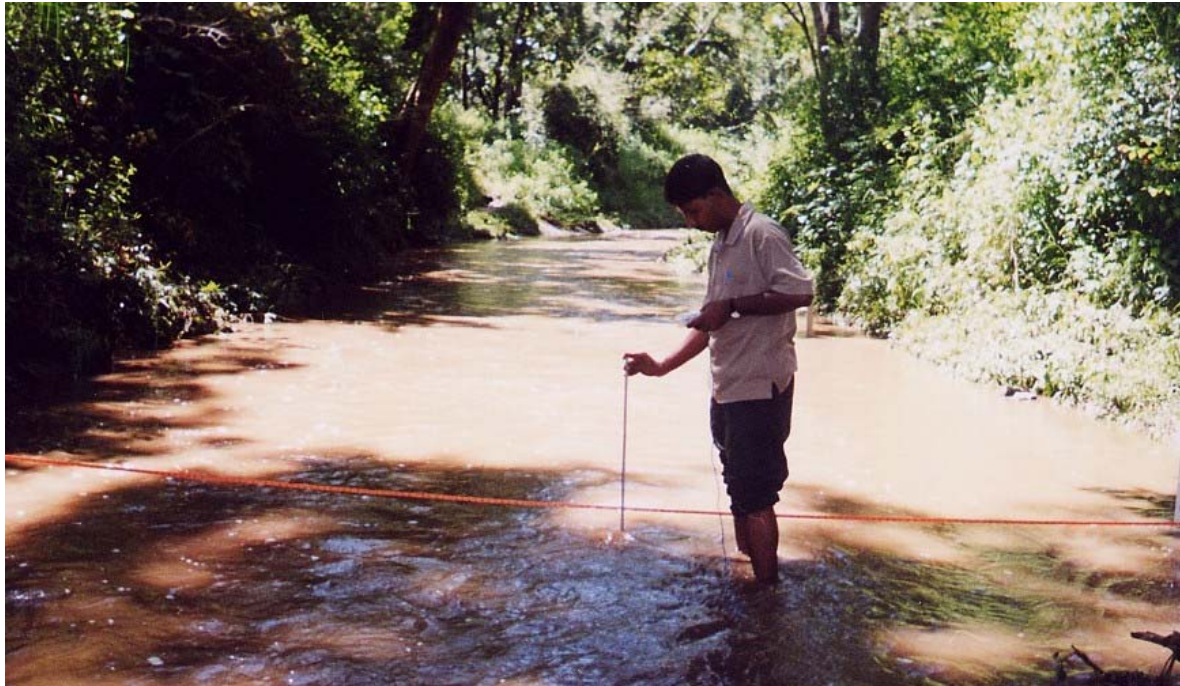
Figure 3-28. Taking current meter readings in Soreda control catchment
