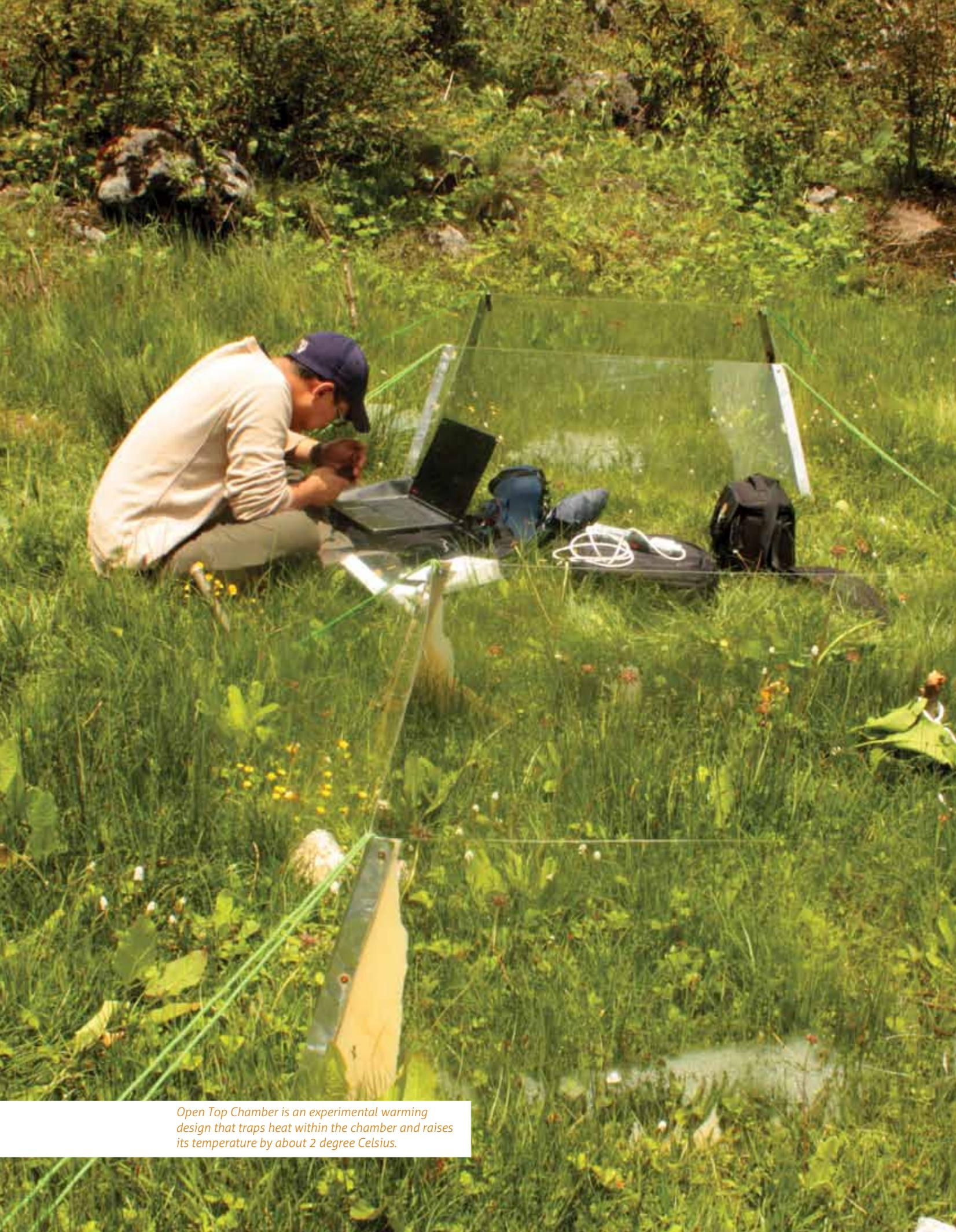
*Open Top Chamber is an experimental warming design that traps heat within the chamber and raises its temperature by about 2 degree Celsius.*
